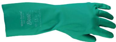
Nitri-Solve Waterproof Glove is made of 15 mil nitrile with flock lining. A good choice when handling harsh cleaners, petrochemicals, oils and greases. Specify small, medium, large or extra large by add S, M, L or XL after the stock number.
